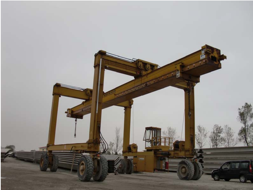
Precast yard transporter 250 t in Pontetaro (ITA)
