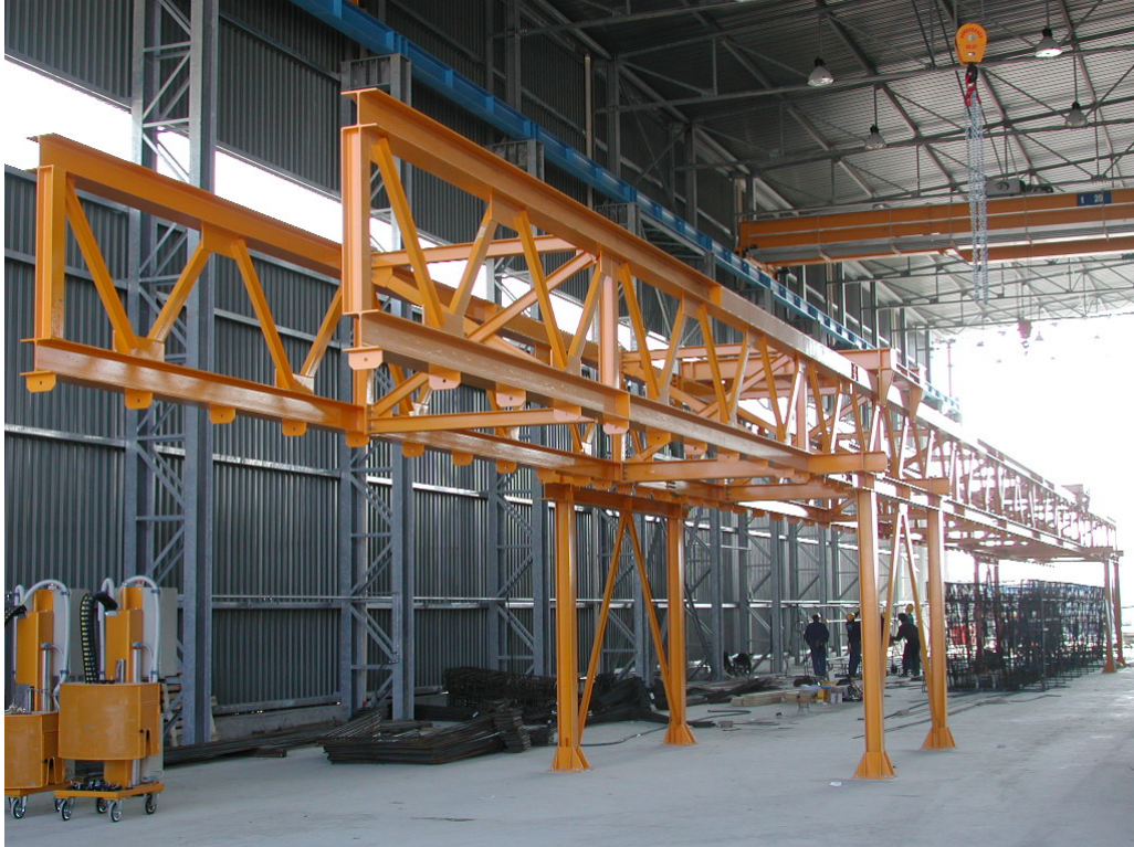
Rebar cage lifter Italian HSR – Milano-Bologna jobsite (ITA)
