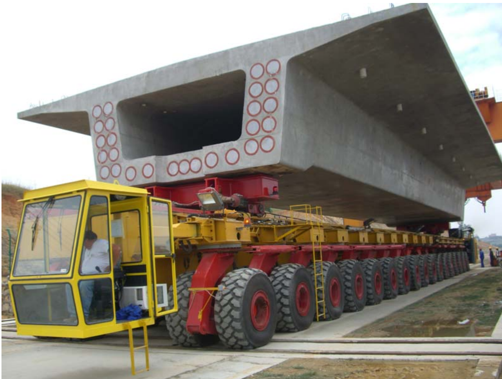
Tyre carrier 950 t in JingJang (PRC)
